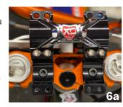
b) If your kit came with nylon lock nuts and washers, install the top clamp with all eight of supplied 20mm long bolts and snug down the MAKO360 top clamp. Tighten the perch bolts.
